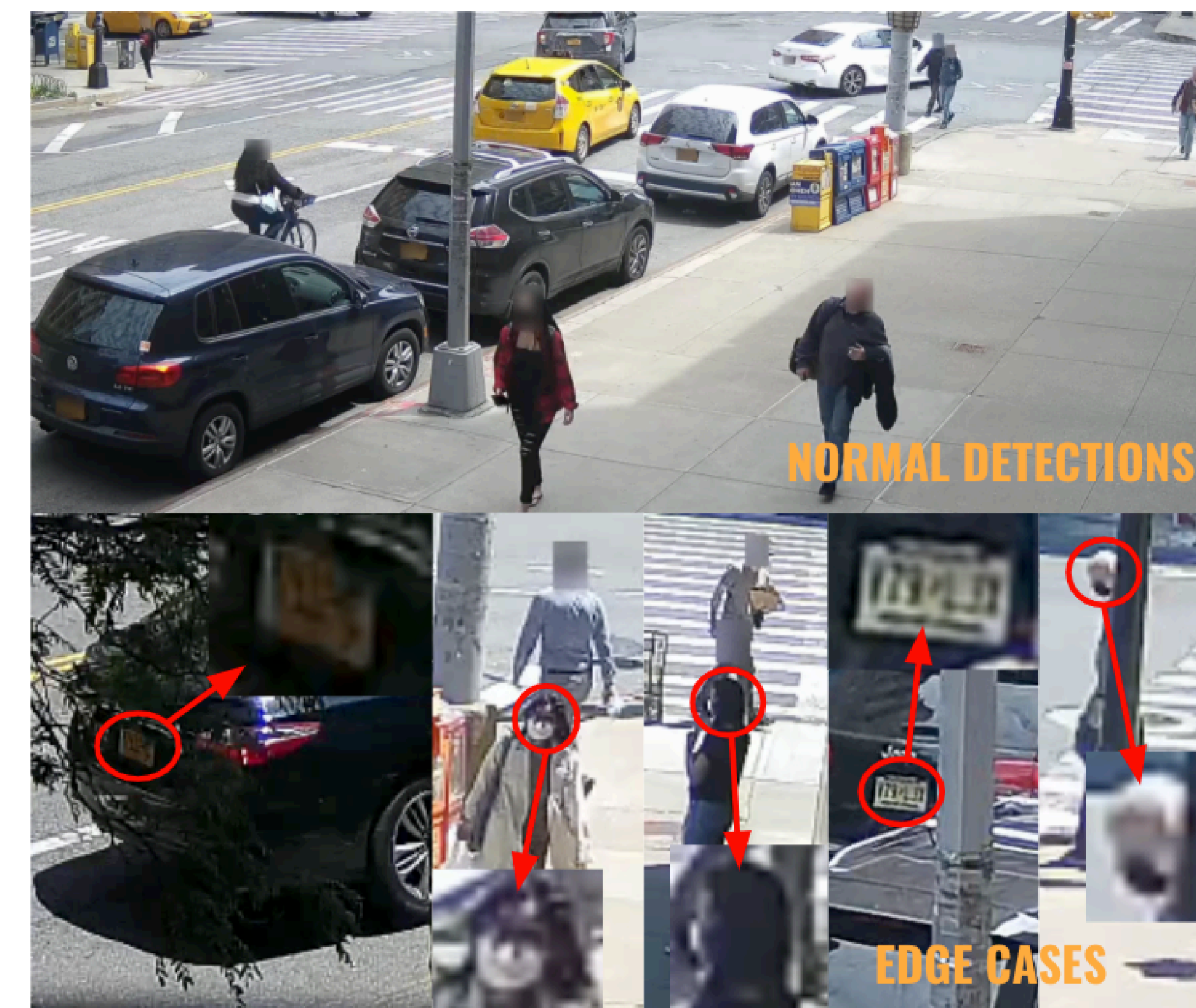
Figure 4: Successful detection and blurring of faces and license plates (top). False negatives highlighted in various edge cases (bottom).
