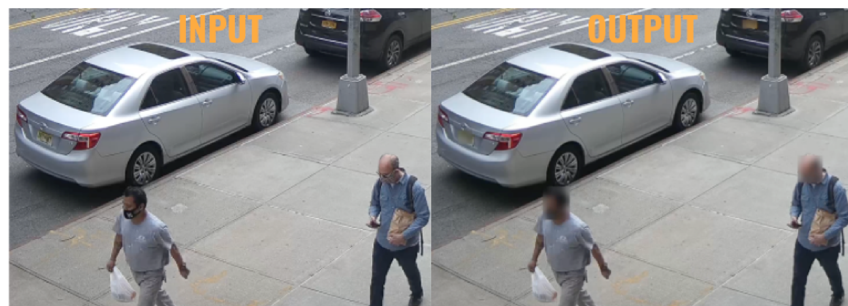
Figure 1: Example input (raw unblurred frame) and output (frame with faces and licenses blurred).
