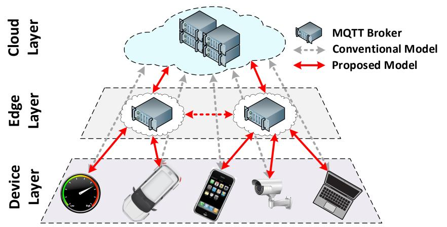
Moving MQTT brokers to distributed edges
